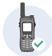
Phone will display 'searching for network' and then 'Registered', which typically takes 30-60 seconds. If phone has been left on when inside of a building, it will take longer to find and register with the network in order to save power. To accelerate network registration, turn phone off and on once outside.
