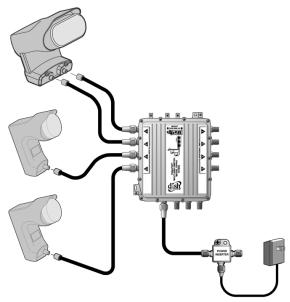
Figure 6. DISH Pro Plus 44 Connections
