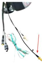
The GPS connection is optional if the tracking function is not required. If connected, and tracking is enabled, position or location information will be shown on your tracking messages and alert messages.
