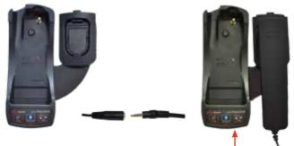
Privacy Handset mode is enabled when the handset is removed from the cup. Please ensure to re-dock the Privacy Handset when not in use.
