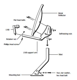
For camping combos the Mounting foot and mast are replaced with a tripod.
